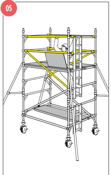
Fit 2 more diagonals in opposite directions between the 3rd and 5th rungs of the tower. Fit a trapdoor deck on the 4th rungs of the tower with the trapdoor next to the ladder and opening towards the outside of the tower.
