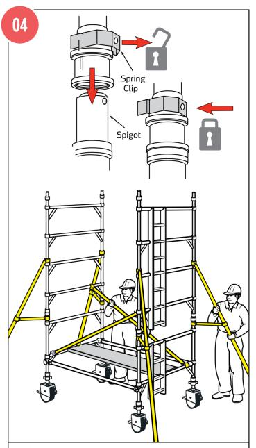
Fit 2 additional end frames and check the frame interlock clips are engaged. Fit 2 diagonal braces in opposing directions between the 1st and 3rd rungs. Ensure the frames are vertical and level by checking with a spirit level and setting the adjustable legs as required.
