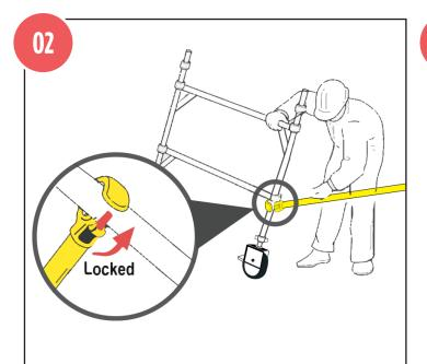
Fit one horizontal brace (red) onto the vertical of the span frame, just above the bottom rung, with the claw facing outwards. The frame will now be self-supporting.
