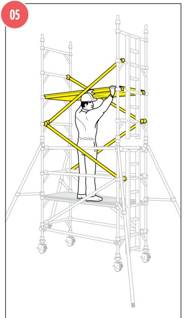
Fit 2 pairs of diagonal braces in opposing directions between the 3rd and 5th rungs and the 5th and 7th rungs.
