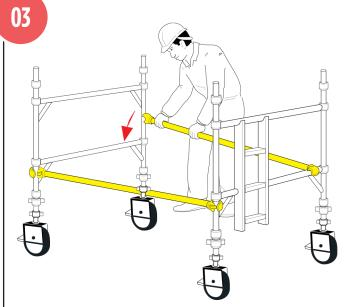
Position the ladder frame as shown and fit the other end of the horizontal brace onto the vertical, just above the bottom rung. Fit a second horizontal brace between the bottom rungs on the other side of the frames to square the tower.
