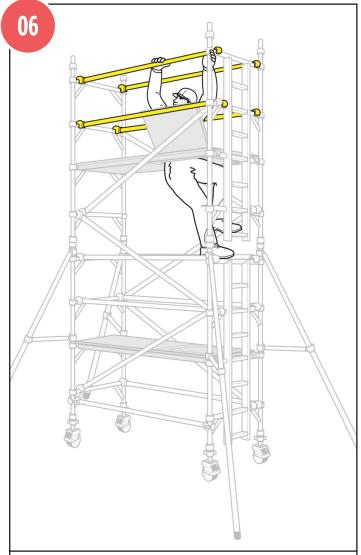
Climb up the inside of the tower and from the protected position of the trapdoor, fit guardrails to the 7th and 8th rungs (in that order) on both sides of the tower.
