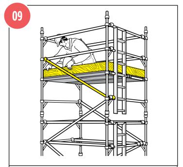
Repeat the previous steps until the required height of tower is reached. Fit a single diagonal at the top of the tower as shown. Fit the toeboards.
