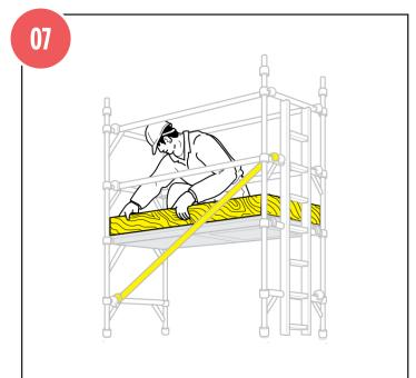
Continue the procedure until the required working height is reached, adding additional pairs of end frames, diagonal braces and fitting trapdoor platforms, as shown on previous steps. At every platform level, add horizontal braces as guardrails from the protected position within the trapdoor, (as shown in step 5).
