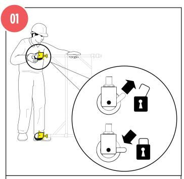
Push castor onto adjustable leg to secure. Insert 2 adjustable leg/castor assemblies into span frame. Base plates can be fitted to adjustable legs if it is not necessary to move the tower.
