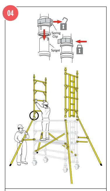
Fit a trap door deck on the 2nd rung with the trapdoor next to the ladder. Fix guardrails on the 3rd and 4th rungs on both sides of the tower.
