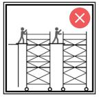
Do not bridge between towers or Please contact Access Towers for information on the correct equipment for Bridging Towers.
