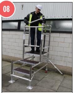
Once the platform is accessed, close the gate behind you; ensure that the clips are engaged and fit the 2 guardrail braces.
