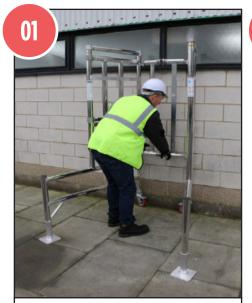
Open the unit on a firm and level base, lock the folding section and then lock the wheels.
