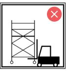
Do not lift the tower with mechanical equipment
