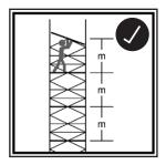
Maximum distance between platforms shall not exceed 2.25m other structures except the distance to the first platform max 3.40m.
