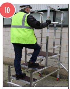
When descending from the platform, use the step platforms and face the folding frame.
